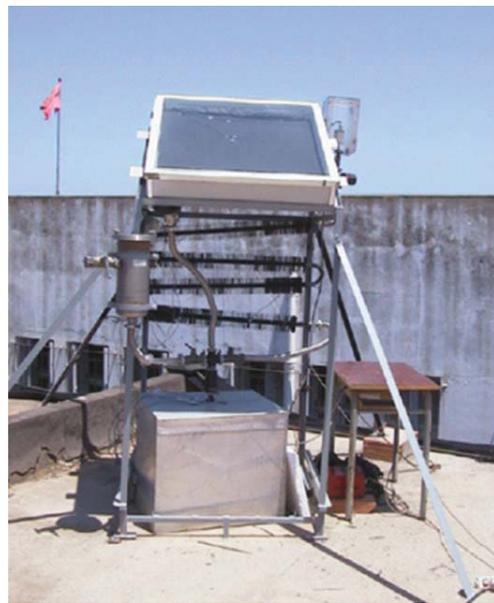
Figure 11. Solar refrigerator tested in Rabat, Morocco [77].
