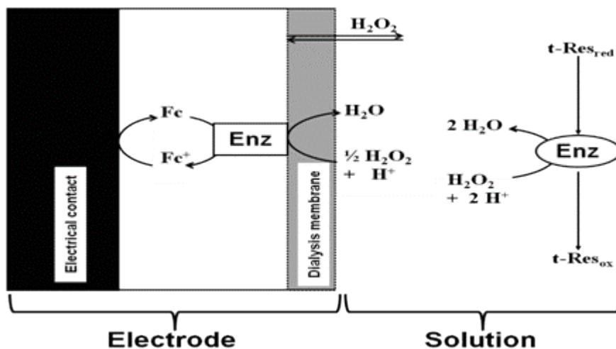
Scheme 1. Schematic representation of the operating principle of the biosensor, (Enz = PBI'S or PBHR).
