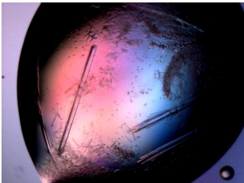
Figure 4. An example of different crystal morphologies found within the same crystallization condition (Hatzopoulos *et al.*, 2008). Plates and needles morphologies are present under the same crystallization condition.
