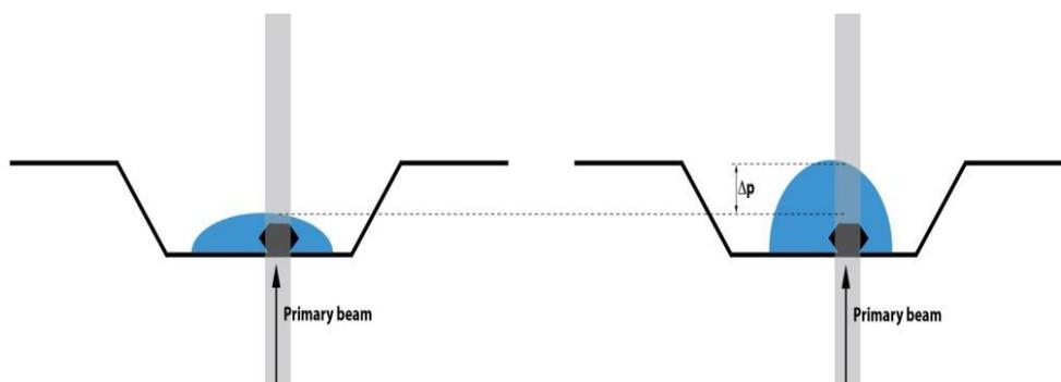
Figure 2. A schematic illustrating the effect of primary beam path in buffer. In the figure above both crystals are of identical diffraction properties. The additional path ( $\Delta p$ ) traversed by the primary beam (grey) through the buffer surrounding the crystal will result in a significant increase in background on the detector. This will then result in an apparent decrease in the  $I/\sigma(I)$  of the data collected.
