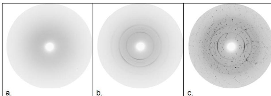
Figure 6. Diffraction patterns obtained on EMBL X13 beamline using a prototype *in situ* compatible support. a) air (control) b) using EMBL prototype sandwich plate without crystal c) EMBL sandwich plate including diffraction from lysozyme crystal. The thin 4 $\mu$ m film material within the beam path limits the presence of background to 2 faint rings.
