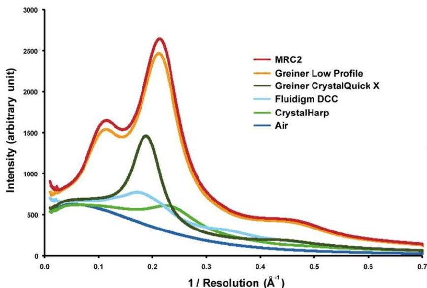
Figure 5. Levels of X-ray background measured for different crystallization plates (reproduced with permission from Bingel-Erlenmeyer (2011)). The best performing plates are the Fluidigm Diffraction Capable Chip and Crystal Harp that achieve background absorbance's levels close to that of air alone.
