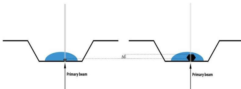
Figure 3. A schematic representation of the effects of crystal volume on diffraction intensity. The crystals in the images above are of identical diffraction properties. However, the volume illuminated by the primary beam is significantly different. This will result in a significant differences in diffraction intensity recorded between the two examples.
