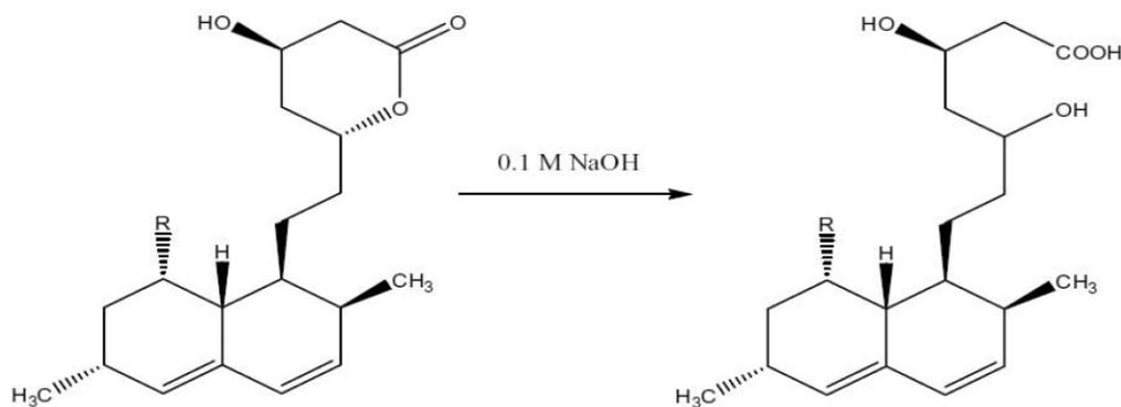
Figure 2. Transformation of a hydroxy acid form of monacolin K from the corresponding lactone form upon alkalization (0.1 M NaOH).
