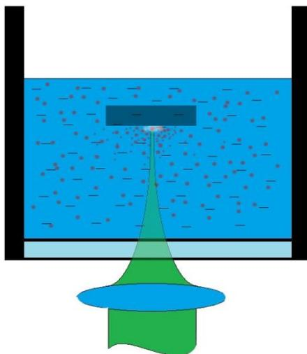
Figure 5. The scheme of laser exposure of metallic target in aqueous solution of Uranil-chloride.
