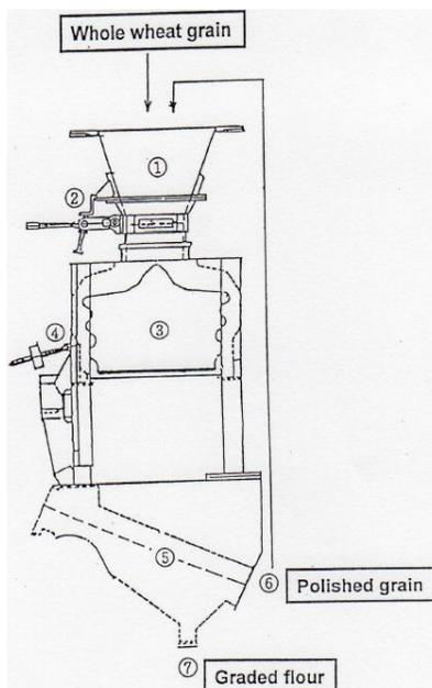
1, Receiver; 2, Lever; 3, Roller; 4, Controller; 5, Sieve; 6, Outlet for polished grain; 7, Outlet for graded flour.
