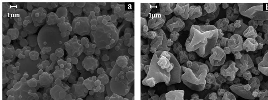
Figure 2. SEM pictures of powders dried from water/IPA 7/3 v/v systems containing: a) GISO3; b) GISO3-Leu15.
