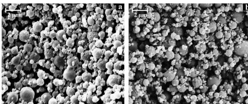
Figure 5. SEM images of GAP microparticles obtained by SAA at different GS/alginate/pectin ratio: GAP1 (a) and GAP4 (b).
