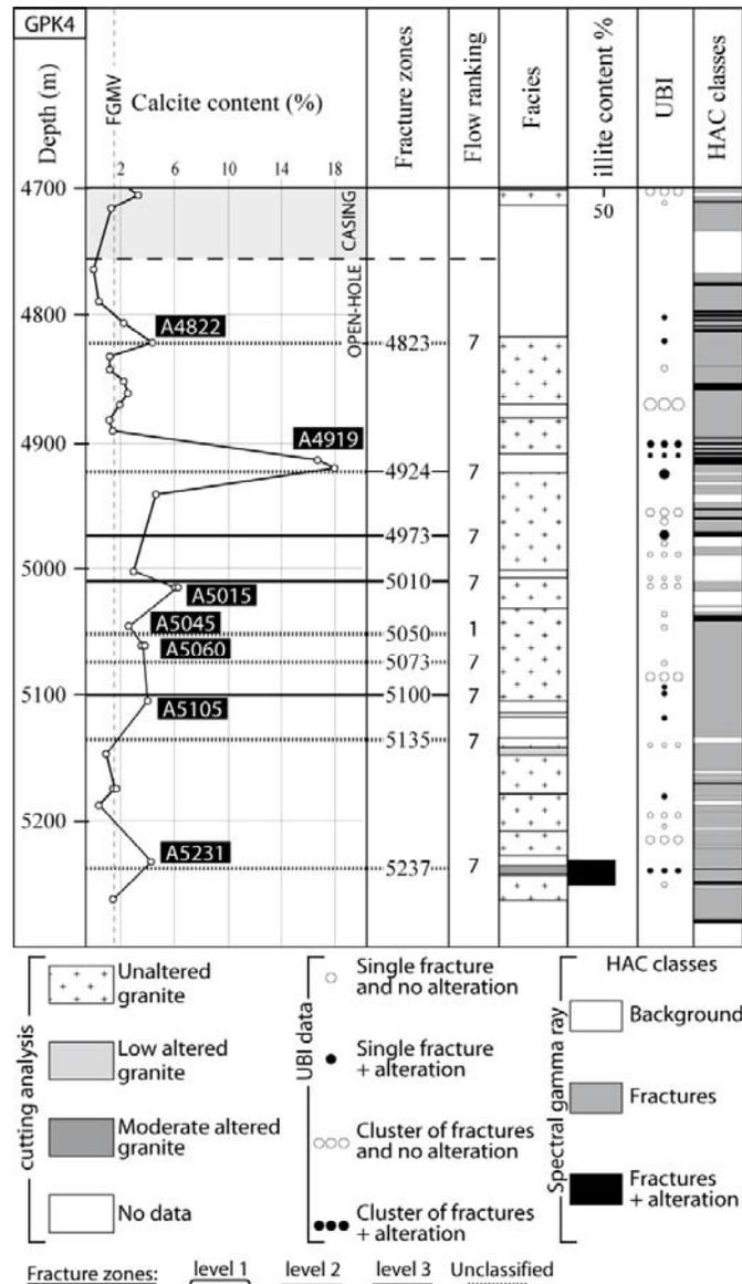
Figure 6. GPK4 open-hole synthetic log (modified after Hébert et al., 2010). Fracture zones (from Gentier et al., 2005; Sausse et al., 2007), flow ranking (from Sausse et al., 2007), petrographic facies and illite content (from Genter et al., 1999). FGMV grey zone corresponds to the fresh granite maximum value of calcite (White et al., 2005).
