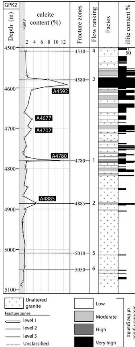
Figure 4. GPK2 open-hole synthetic log (modified after Hébert et al., 2010). Fracture zones (from Gentier et al., 2005; Sausse et al., 2007), flow ranking (from Sausse et al., 2007), petrographic facies and illite content (from Genter et al., 1999). FGMV grey zone corresponds to the fresh granite maximum value of calcite (White et al., 2005).
