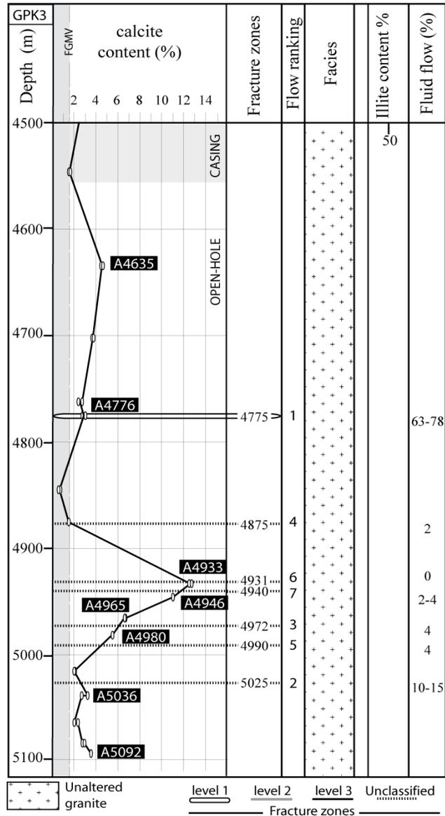
Figure 5. GPK3 open-hole synthetic log (modified after Hébert et al., 2010). Fracture zones (from Gentier et al., 2005; Sausse et al., 2007), flow ranking (from Sausse et al., 2007), petrographic facies and illite content (from Genter et al., 1999). FGMV grey zone corresponds to the fresh granite maximum value of calcite (White et al., 2005).
