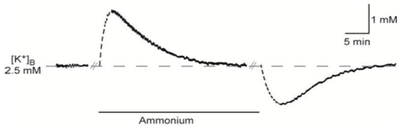
Figure 10. Shown is a calculated trace resulting from the correction of the  $NH_4^+$ -mediated voltage signal of the ion sensor, revealing the estimated change in  $[K^+]_o$ . Wash-in and wash-out phase of  $NH_4^+$  are dotted to emphasize that  $NH_4^+$  concentrations change and calculations may not be accurate during these periods.
