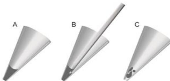
Figure 1. Schematic drawing of the tip of the ion-selective channel after its filling. (A) If the sensor is filled in properly, it forms a concave surface against the backfill. (B) Touching the sensor while backfilling it, might destroy its surface. (C) In a poorly silanized microelectrode, the sensor retracts from the inner capillary wall and may form several spheres.
