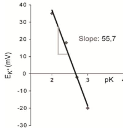
Figure 5. Plot of  $E_{K^+}$  against the logarithm to the base ten of the potassium concentration (pK) and a linear fit of the data. The slope of this fit is 55.7 mV.
