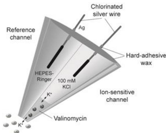
Figure 2. Schematic drawing of a double-barreled, potassium-sensitive microelectrode after its filling. For illustration purposes, the electrode is shown untwisted. The sensor barrel is filled with a liquid neutral  $K^+$  carrier based on valinomycin and backfilled with 100 mM KCl. The reference barrel is filled with HEPES-buffered saline (“HEPES-Ringer”). Chlorinated silver wires are inserted into both channels and each barrel is sealed with dental wax.
