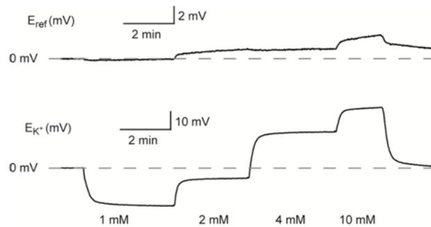
Figure 4. Typical calibration of a potassium-selective microelectrode in the experimental chamber. Shown are traces of the voltage-responses of the reference channel ( $E_{ref}$ , upper trace) as well as of the ion-selective channel ( $E_{K^+}$ , lower trace) in response to stepwise changes in the potassium concentration in the perfusion saline from a basic level of 2.5 mM K<sup>+</sup> (defined as “zero”/ 0 mV) to 1, 2, 4, and 10 mM K<sup>+</sup> as indicated above.
