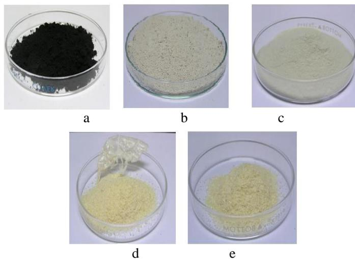
Figure 7. The adsorbents of Activated carbon (a), Bentonite 150 (b), Bentonite 200 (c), Chitin (d) and Chitosan (e).
