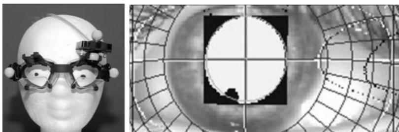
Figure 1. Left panel: Lightweight, monocular EyeSeeCam. Right panel: Extracted pupil center and overlaid eyeball model.
