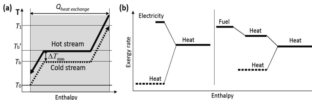
Figure 1. Principle of exergy recovery: (a) basic concept of exergy recovery, (b) two examples of how to elevate the exergy rate.
