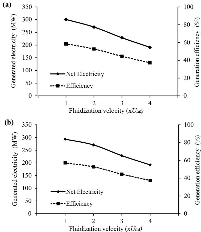
Figure 6. Effect of the fluidization velocity on the generation of electricity and generation efficiency (SCWG pressure of 25 MPa): (a) turbine inlet temperature of 1500°C, (b) turbine inlet temperature of 1300°C.
