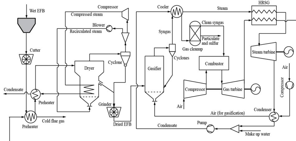
Figure 8. Schematic diagram of the integrated power generation system for EFBs covering drying, gasification, and combined cycle.
