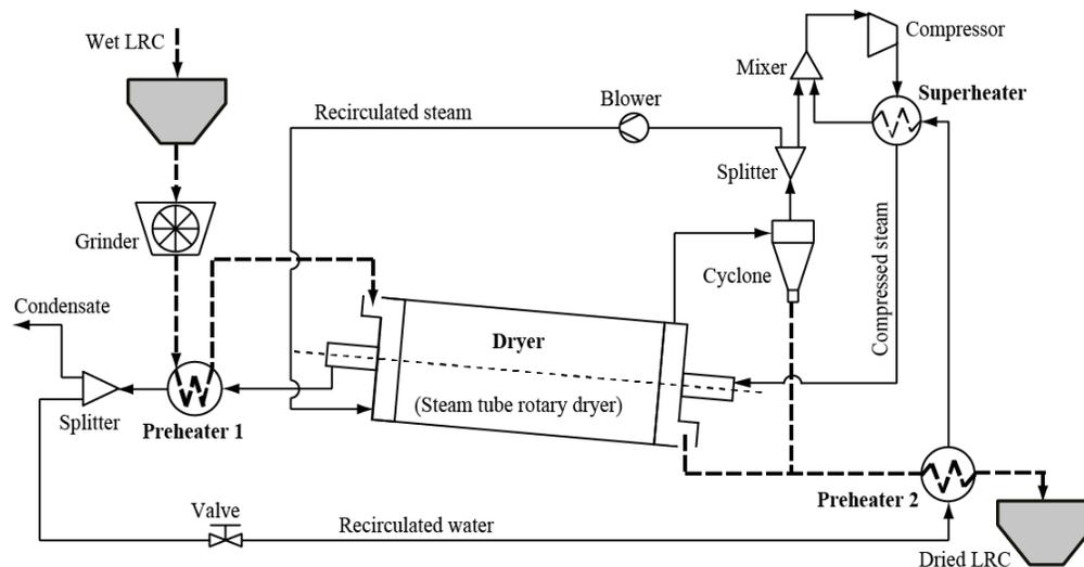
Figure 2. Process flow diagram of the proposed drying of LRC based on EPI.
