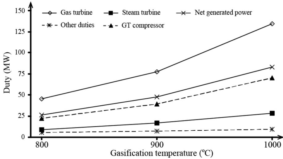
Figure 9. Simulation results of the integrated power generation from EFBs based on EPI versus the gasification temperature.
