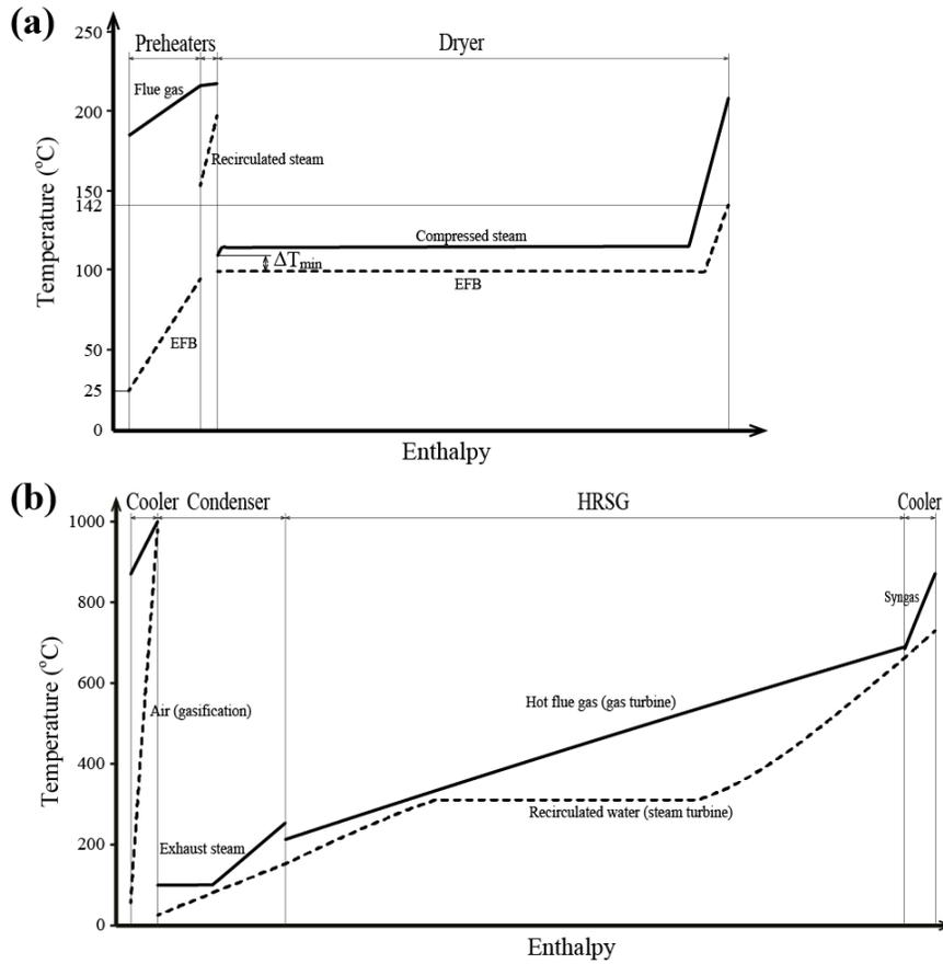
Figure 10. Temperature–enthalpy diagram of the integrated power generation from EFBs: (a) drying, (b) gasification and combined cycle (gasification temperature of 1000°C).
