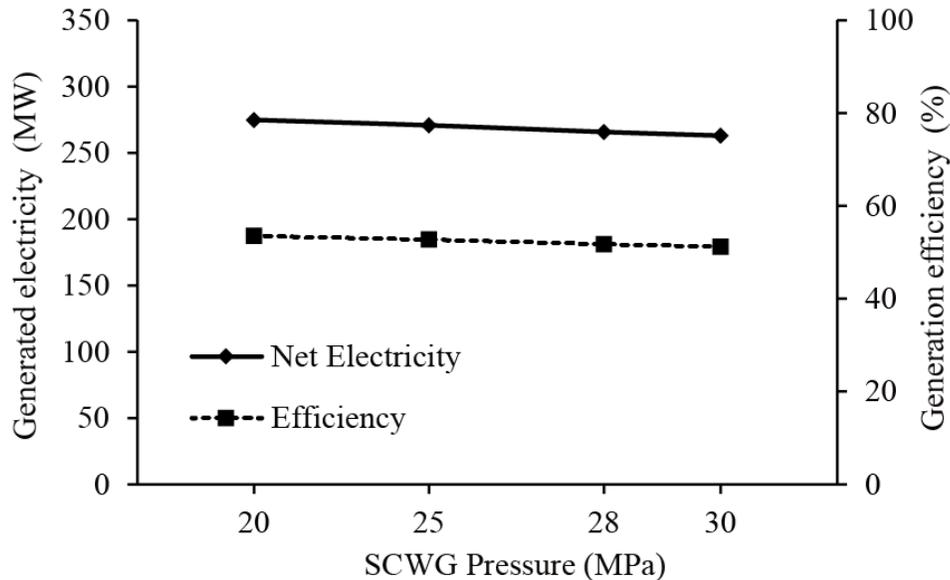
Figure 7. Effect of SCWG pressure on the generated electricity and generation efficiency (turbine inlet temperature and fluidization velocity are 1500°C and  $2 U_{mf}$ , respectively).
