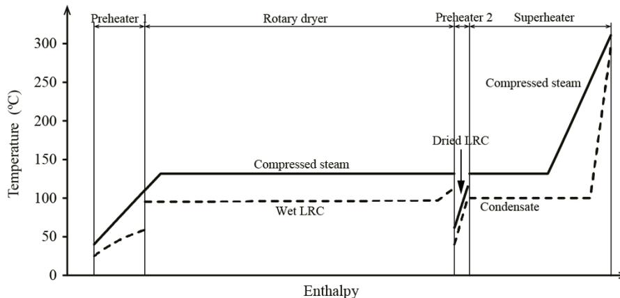
Figure 4. Temperature–enthalpy diagram of the proposed LRC drying.
