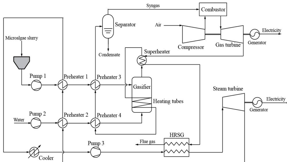
Figure 5. Basic process flow diagram of the integrated SCWG and combined cycle for microalgae.
