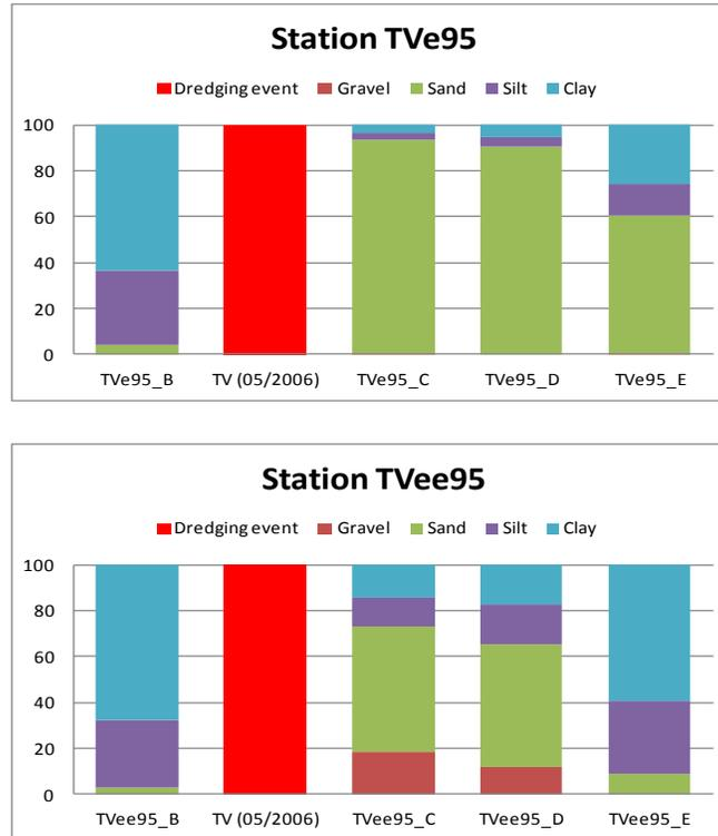
Figure 5. TV site: more intensely dredged area. As early as five months after dredging, sediments show unimodal distributions, with significant contents of coarse fractions (samples Tve95C and TVee95C).
