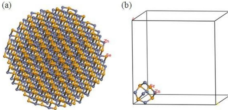
Figure 1. Nanocrystal structure of semiconductor: (a) schematic of a nanocrystal sphere of ZnSe; (b) the crystal-cage of ZnSe with only surface atoms.
