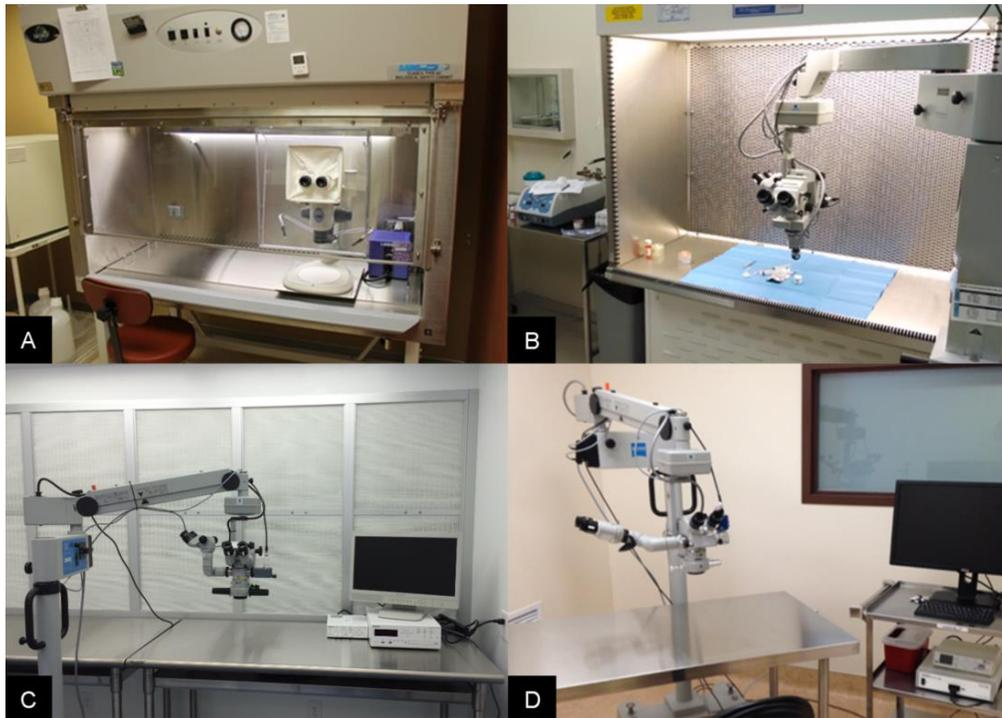
Figure 1. A) Dissecting microscope set up in a vertical laminar ISO 5 flow hood with biosafety shield (courtesy Minnesota Lions Eye Bank). B) Operating microscope set up in a large ISO Class 5 horizontal laminar flow hood (courtesy Iowa Lions Eye Bank). C) Operating microscope set up in ISO Class 5 work zone inside at tissue processing room (courtesy Georgia Eye Bank). D) Operating microscope set up in an ISO Class 5 clean room (Lions VisionGift).
