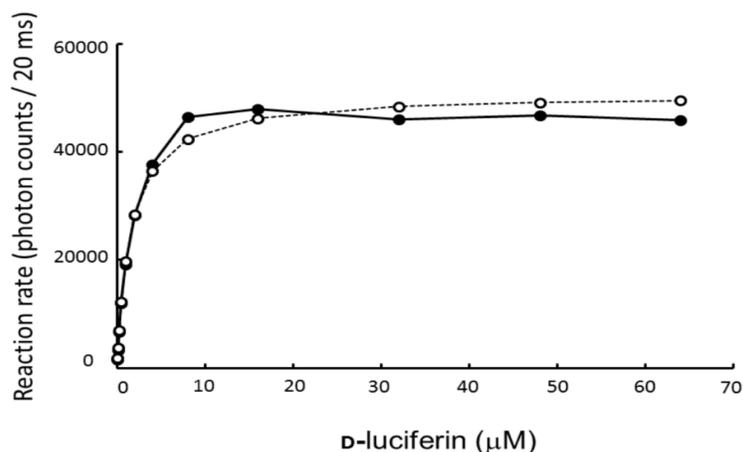
Figure 3. Determining  $K_M$  of luciferase for luciferin. The reaction rate (ordinate), which was estimated by the number of photon counts in 20 ms time gates, was plotted relative to the input luciferin concentration (abscissa). Closed and open circles show measured and expected values, respectively. Data are shown as the mean  $\pm$  SD ( $N = 6$ ).
