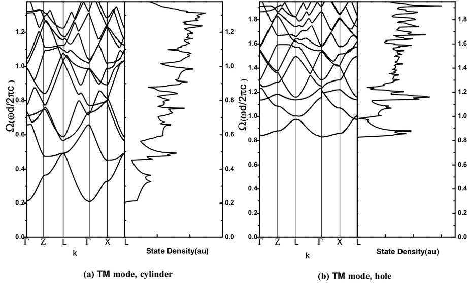
Figure 9. Band structures and DOS of the TM modes. a) 2D M/D cylinder ( $\varepsilon_\infty = 1, \varepsilon_2 = 2$ ) b) hole ( $\varepsilon_\infty = 1, \varepsilon_1 = 2$ ) PCs with  $R/d = 0.2, d/b = 0.9, \Omega_p = 1$ .
