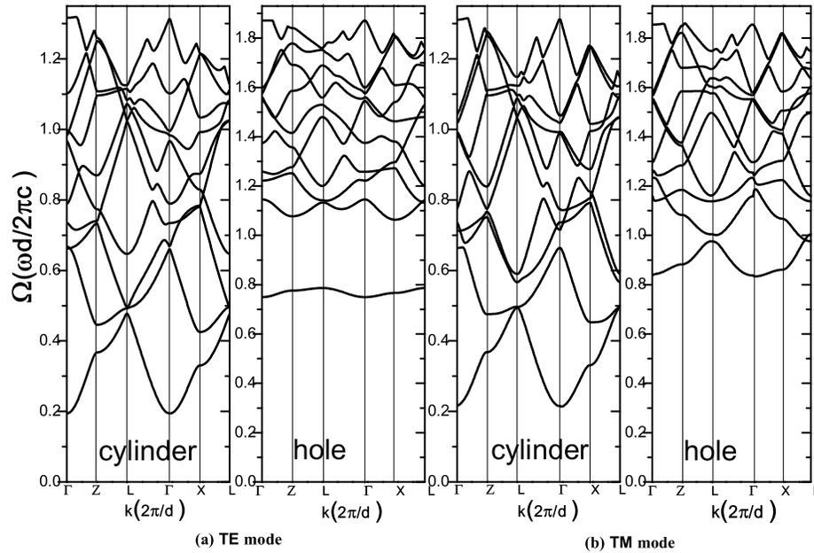
Figure 10. Band structures of the eigen modes for the 2D M/D square pillar, ( $\varepsilon_\infty = 1, \varepsilon_2 = 2$ ) and hole ( $\varepsilon_\infty = 1, \varepsilon_1 = 2$ ) PCs with  $a/d = 0.2\sqrt{\pi}, d/b = 0.9, \Omega_p = 1$ . a) TE modes. b) TM modes.
