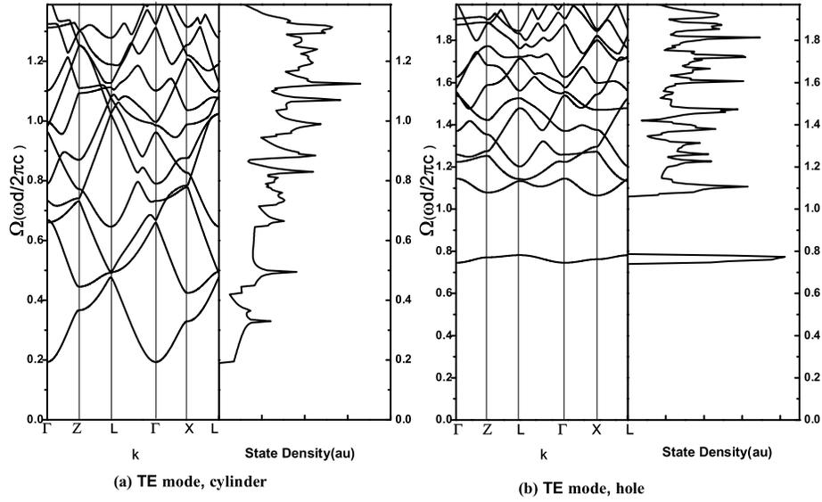
Figure 8. Band structures and DOS of the TE modes. a) 2D M/D cylinder ( $\varepsilon_\infty = 1, \varepsilon_2 = 2$ ) b) hole ( $\varepsilon_\infty = 1, \varepsilon_1 = 2$ ) PCs with  $R/d = 0.2, d/b = 0.9, \Omega_p = 1$ .
