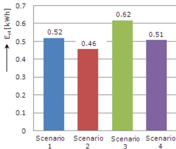
Figure 10. Electricity consumption of the FCUs from the HRU and FCUs system.
