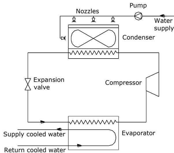
Figure 4. Schematic of the chiller and water mist system.
