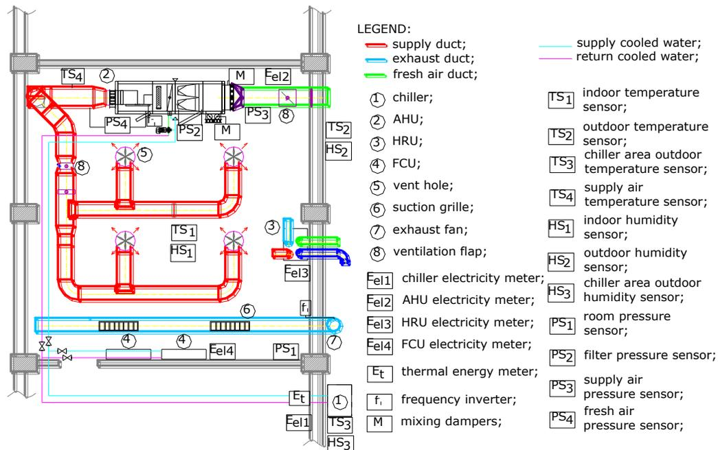
Figure 3. Schematic of the location of the equipment in the experimental room.
