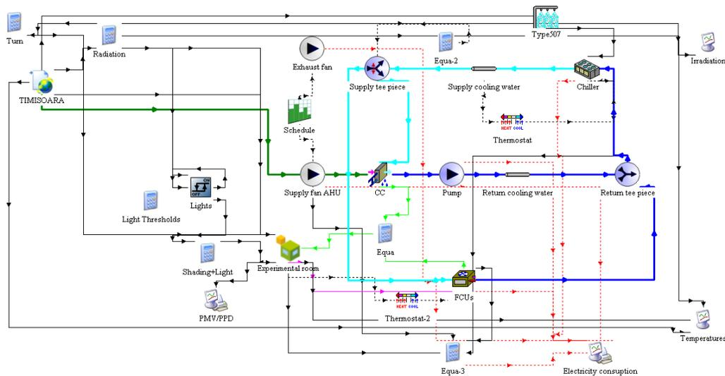
Figure 14. Scheme of the VAC system model built in TRNSYS.
