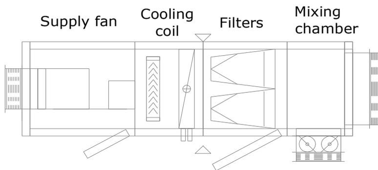
Figure 5. Schematic of the air handling unit.
