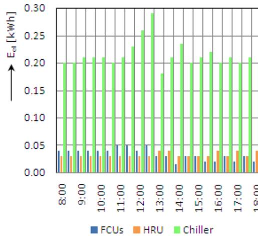
Figure 9. Variation of the hourly electricity consumption of equipment.
